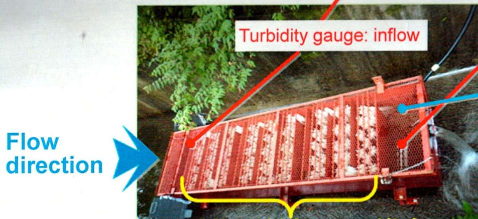
Traps of suspended solid in the river water by non-woven fabric
