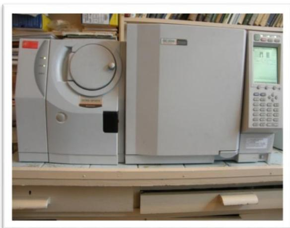
GC-2010 chromatograph and GCMS-QP2010S mass spectrometer
